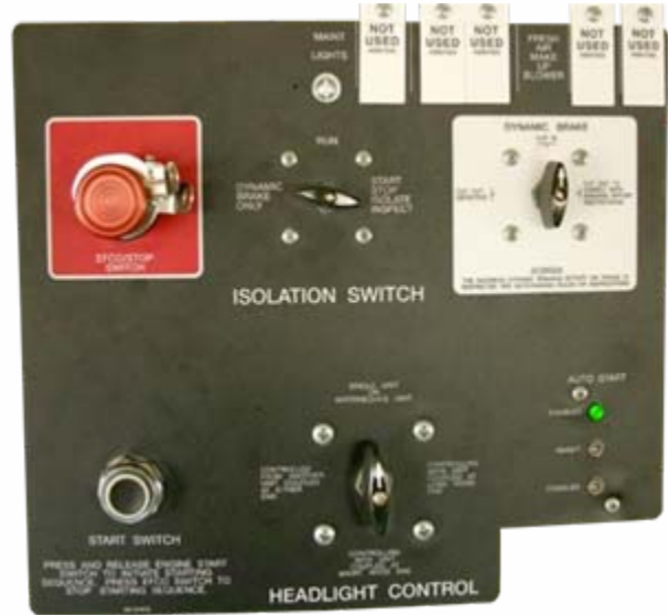
Photo depicts the AESS status portion of the engine control panel.
